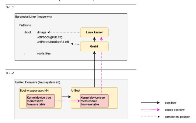
And the booting process of Virtualization solution is as the following diagram:
