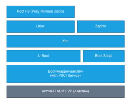
The diagram below gives an overview of the components and layers in the Baremetal Linux stack.
