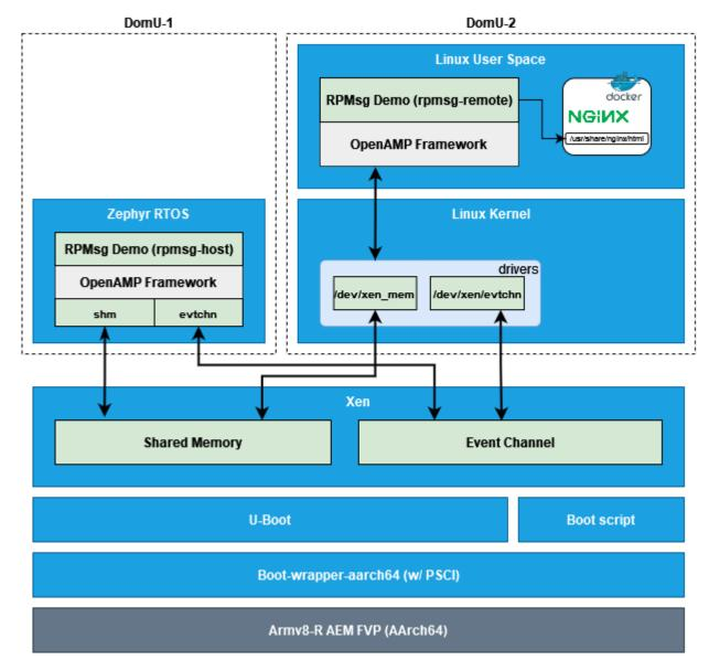
The diagram below gives an overview of the components and layers in the implementation of Virtualization stack.
