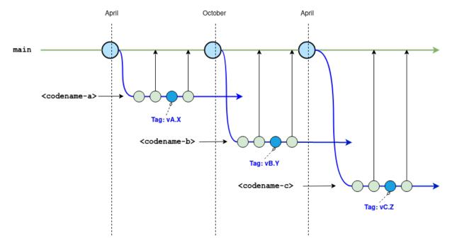
The stack's branch and release process will follow the Yocto release process. Below is a detailed description of the branch strategy for this stack's development and release process.
