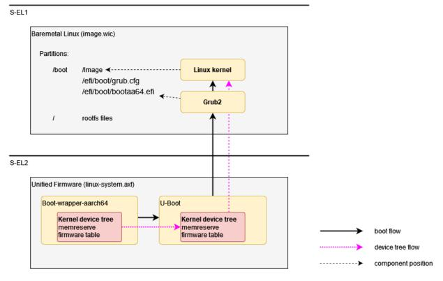
And the booting process of virtualization solution in this stack is as the following diagram:
